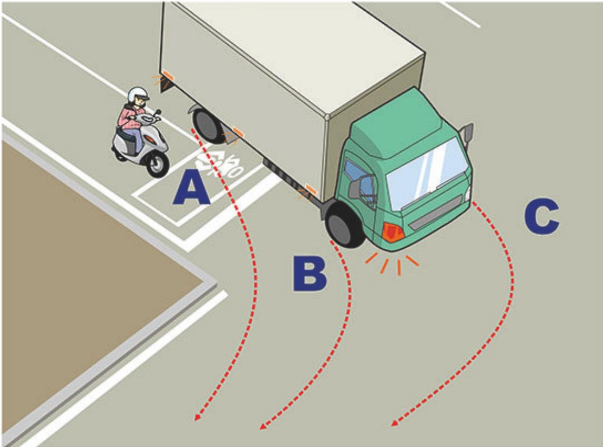
( 2 ) According to the diagram, when a large vehicle makes a right turn, the motorcyclist shall avoid entering which of the following zones due to the difference in the turning radius?
