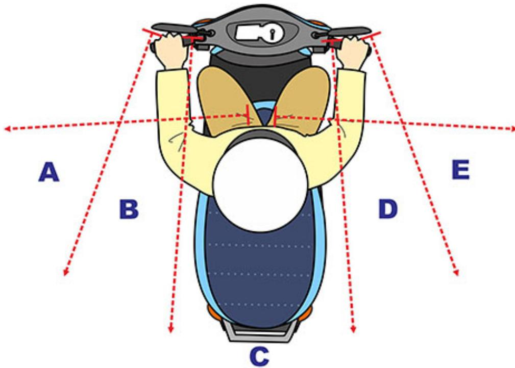
( 1 ) According to the diagram, when the motorcycle is heading straight, which zones cannot be seen by the rider through the side mirrors?
